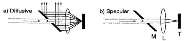
FIG. 5. Hole vignetting when mirror ( $M_2$ ) is close to the lens ( $L_1$ ) of target ( $T$ ). (a) For a diffusively scattering target the vignetting is not substantial and is roughly independent of target position. (b) For a specularly reflective target oriented normal to the illuminating beam the vignetting is complete when the target is at the focal point of the lens. An astigmatic lens would not significantly reduce hole vignetting when the mirror is close to the lens.
