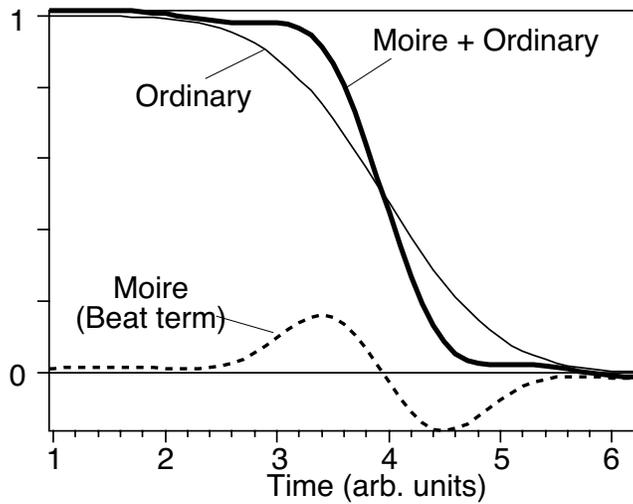
**Figure 4.** Numerically simulated results of conventional and heterodyning measurements, for the case of a perfectly sharp step function input signal and a detector having a Gaussian blur. The thin curve is the conventional result. The use of sinusoidal modulation creates a beat signal (dashed). This is added to the conventional signal to form a composite signal (bold) which has about twice as fast risetime.
