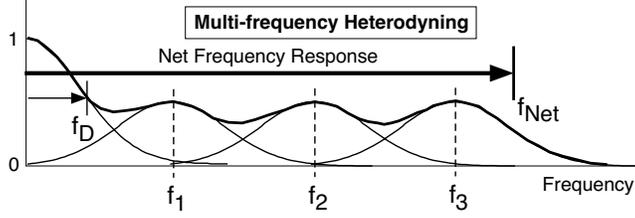
**Figure 6.** Frequency response when  $K$  multiple modulating frequencies ( $f_1, f_2, f_3$ ) are employed in parallel. The net frequency response  $f_{net}$  is boosted over the conventional frequency response ( $f_D$ ) by a factor  $\Psi = f_{Net}/f_D \sim (2K + 0.5)$ .
