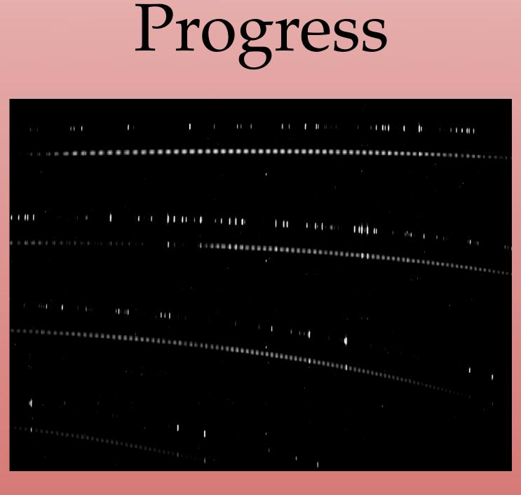
We achieved first light and fringes on Dec. 29, 2007. Our preliminary data analysis pipeline (using only 1 of 5 spectral orders) produces intra-night stability of ~60 m/s after correcting for instrument drifts, and 12 m/s on our reference lamp. We have modified our observing technique for our May '08 observing run, and anticipate at least a factor of 2 improvement in the short term.
