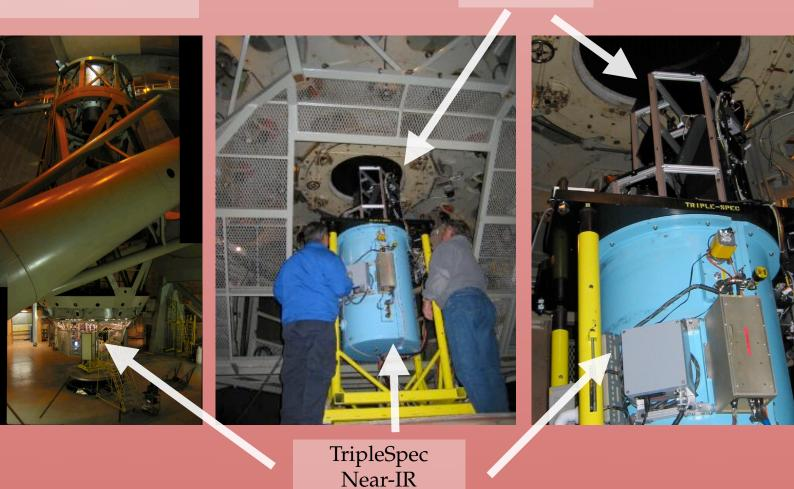
A fixed-delay interferometer superimposes a fine, usually unresolved pattern of fringes on starlight before passing it on to the TripleSpec spectrometer.
