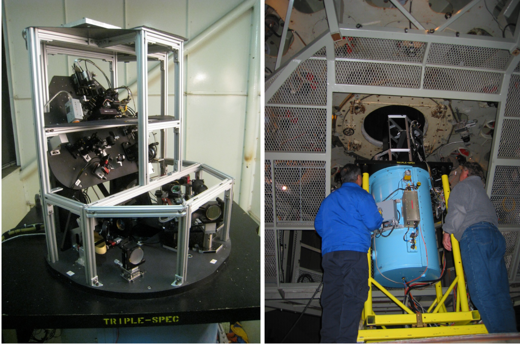
Figure 4. Photograph of the TEDI interferometer, which sits atop Cornell's TripleSpec spectrograph (blue cryogenic cylinder). The interferometer fits in the Cassegrain output cavity of the Mt. Palomar 200 inch mirror, while the TripleSpec is bolted to the bottom of the mirror. The TEDI unit captures the starlight, passes it through an interferometer, and then re-injects it to the spectrograph with a beam having same f/\# and focus location as original beam. (The non-interference spectra displayed in this article are with the arm in place, by summing several fringing exposures to cancel the fringing components.)
