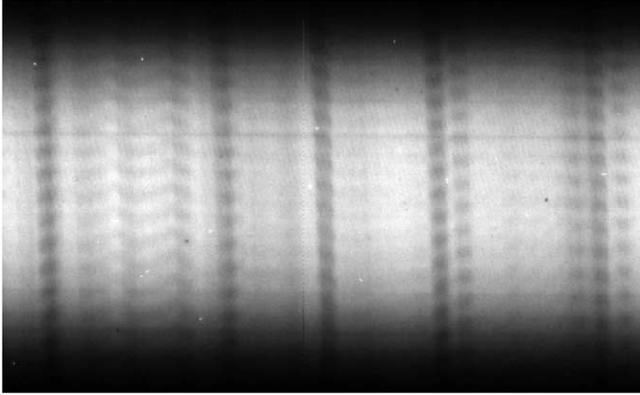
FIG. 1.—Raw fringing spectrum of 51 Peg with iodine, obtained at KPNO on the night of 2002 August 14 (mag 5.5, S/N  $\sim 50$  pixel $^{-1}$ ).
